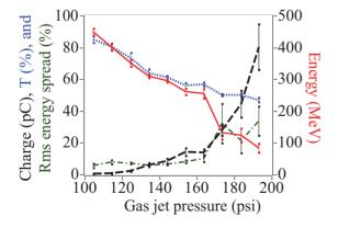
Figure 4: Beam energy (red line, right axis), laser transmission T (blue dotted line, left axis), integrated energy spread (green dash-dot line, left axis) and charge (black dashed line, left axis) as a function of jet pressure for the larger jet.
