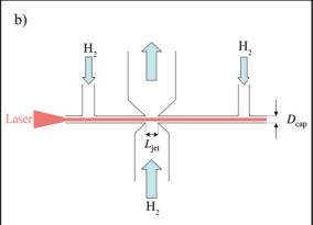
Figure 1: a) The experimental layout used for investigating electron acceleration in a hydrogen-filled capillary discharge waveguide. b) The capillary with embedded gas jet.
